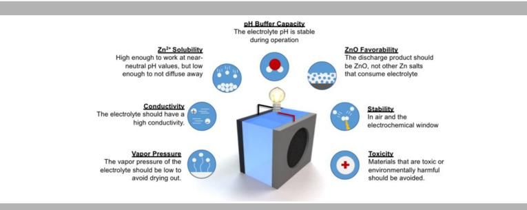
ZAB cell design and components compatibility to solve key bottlenecks of Zn-Air technology by increasing the utilization and rechargeability of Zn electrode, reducing electrolyte poisoning and dry out and increasing the activity and durability of the GDE for the oxygen reduction reaction (ORR) and oxygen evolution reaction (OER) "unlocking" a new 2 electrodes cell design (1 cathode 1 anode).
