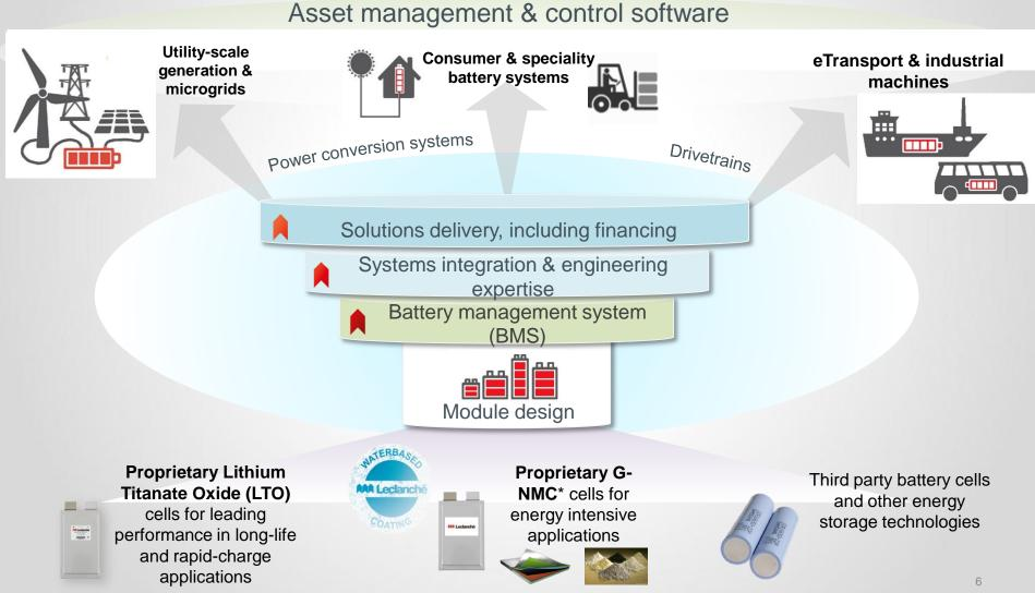
\*Graphite anode and Nickel-Manganese-Cobalt cathode
