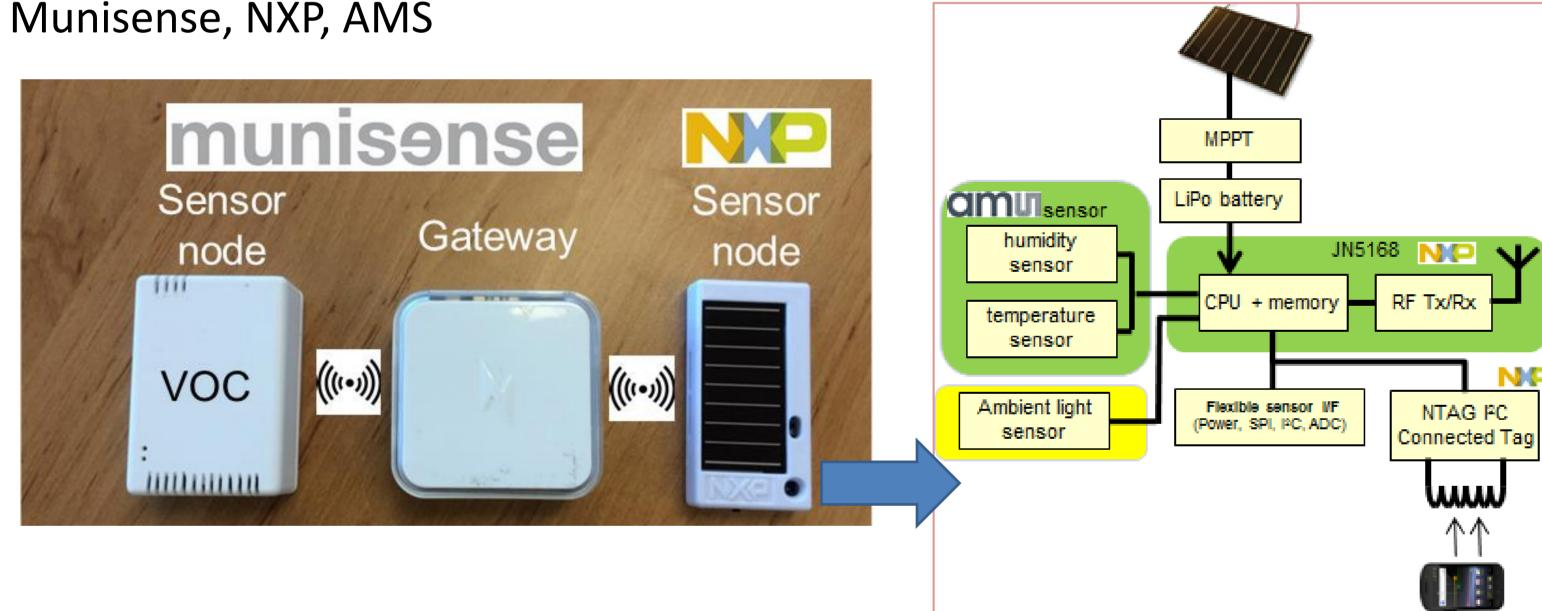
Main Application Fields: CO<sub>2</sub>, temperature and humidity sensors coupled with a web application
